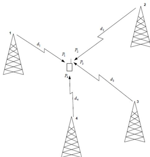
$$T_m = 2 \sqrt{\frac{\sum_{i=1}^N P_i d_i^2}{\sum_{i=1}^N P_i} - \left( \frac{\sum_{i=1}^N P_i d_i}{\sum_{i=1}^N P_i} \right)^2}$$
